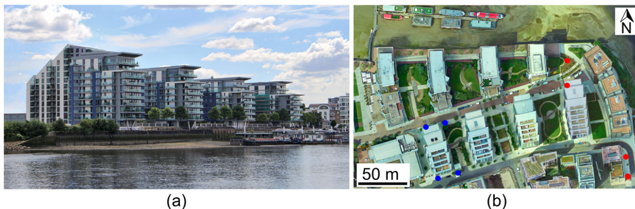
Figure 4.9: (a) Photograph of Wandsworth Riverside Quarter. (b) Aerial image of the site; well locations shown by blue and red circles for cold and warm wells, respectively. Source: Jackson, M. D., Regnier, G., & Staffell, I. (2024). Aquifer thermal energy storage for low carbon heating and cooling in the United Kingdom: Current status and future prospects . Applied Energy , 376, 124096. Modified from IFTech. (2008). Wandsworth Riverside Quarter, London: Borehole drilling and pumping tests . IFTech.
