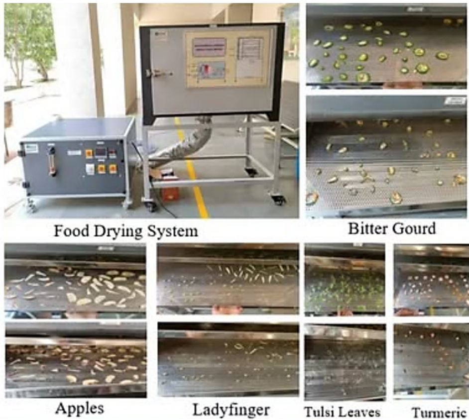
Figure 3.7: Outlet of India's first-ever geothermal water-based food dryer developed by the Centre of Excellence for Geothermal Energy. Source: Bist, N., Yadav, K., & Sircar, A. (2023). Water for food drying: Geothermal energy-based food dryer. In S. Saxena, S. Shukla, & P. K. S. Mural (Eds.), Emerging materials and technologies in water remediation and sensing: Proceedings of ICWT 2022 . Springer.
